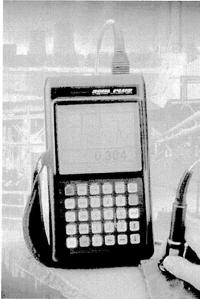
FIGURE 7-63 (c) Thickness gauge on corroded plate.
