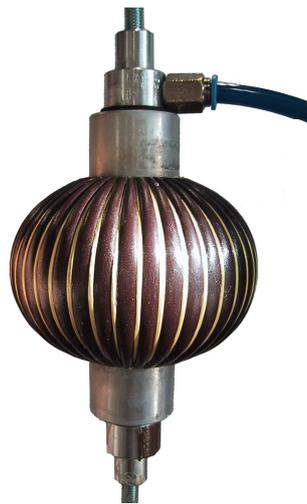
Figure 6: Photograph of inflated state of the second generation PPAM
