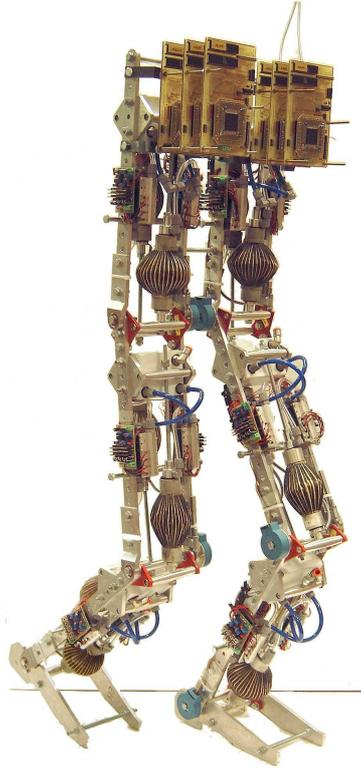
Figure 14: Picture of the robot Lucy, actuated by 12 PPAM
