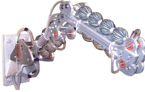
Figure 15: Picture of the manipulator arm, actuated by 4 PPAM
