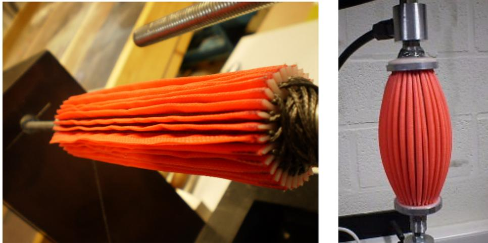
**Figure 3.12:** Photographs of the muscle prototype built with the plastic fabric
