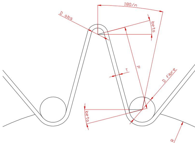
**Figure 3.15:** CAD drawing of the teeth design
