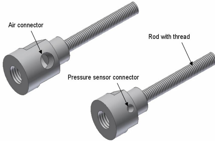
**Figure3.14:** Drawing of the two muscle end connectors
