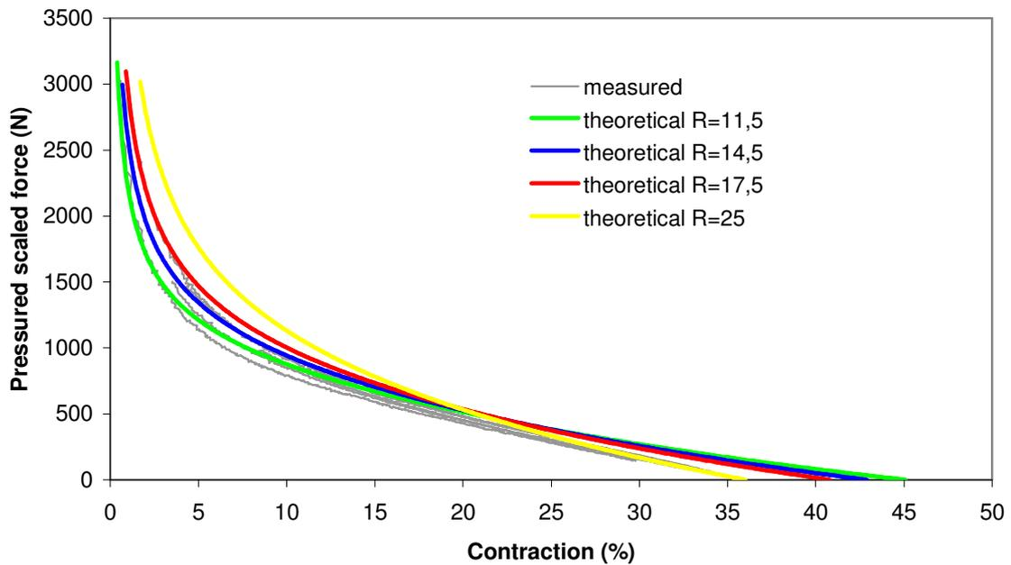
**Figure 3.29:** Pressure scaled measured forces as a function of contraction for 1 muscles made with 32 pleats compared with theoretical model
