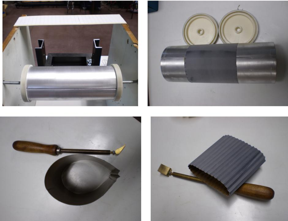
**Figure 3.19:** Photographs of the building and prepleating of the fabric cylinder
