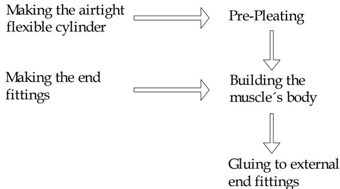
**Figure 3.18:** Diagram of the production process of the third generation of PPAM
