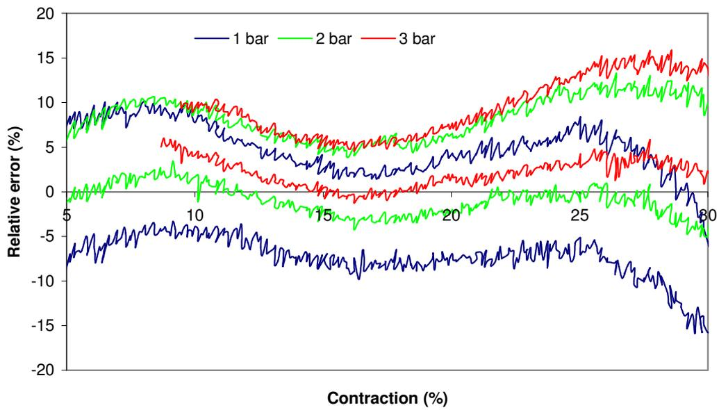
**Figure 3.31:** Relative error between the polinomial fitted estimation and the pressure scaled measured forces as a function of contraction for 1 muscle made with 32 pleats
