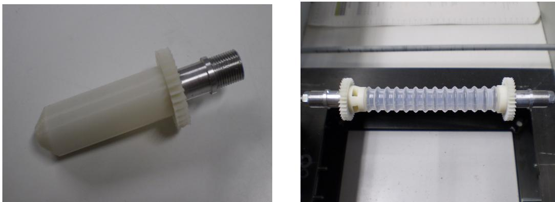
**Figure 3.17:** Photographs of two different implementations to reduce the dead volume
