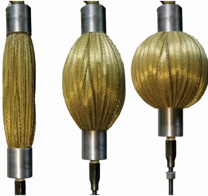
**Figure 3.2:** Photograph of three inflated states of the first generation PPAM
