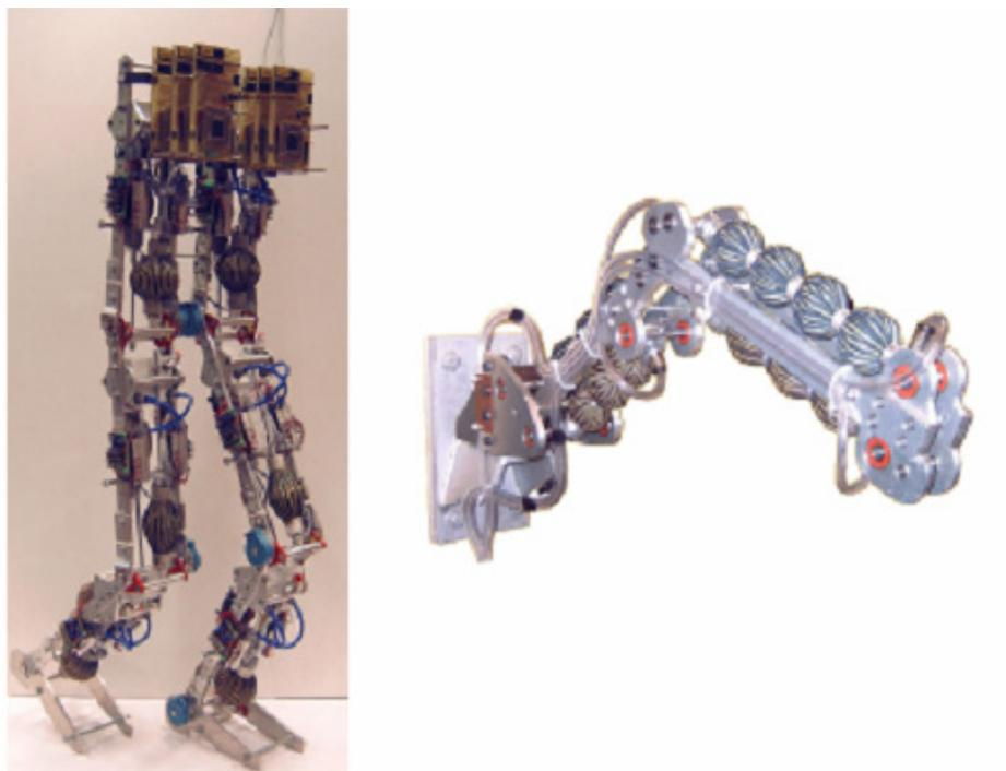
**Figure 1.1:** Photographs of Lucy (bipedal walking robot) and Soft Arm (robotic arm for direct human assistance) [3]
