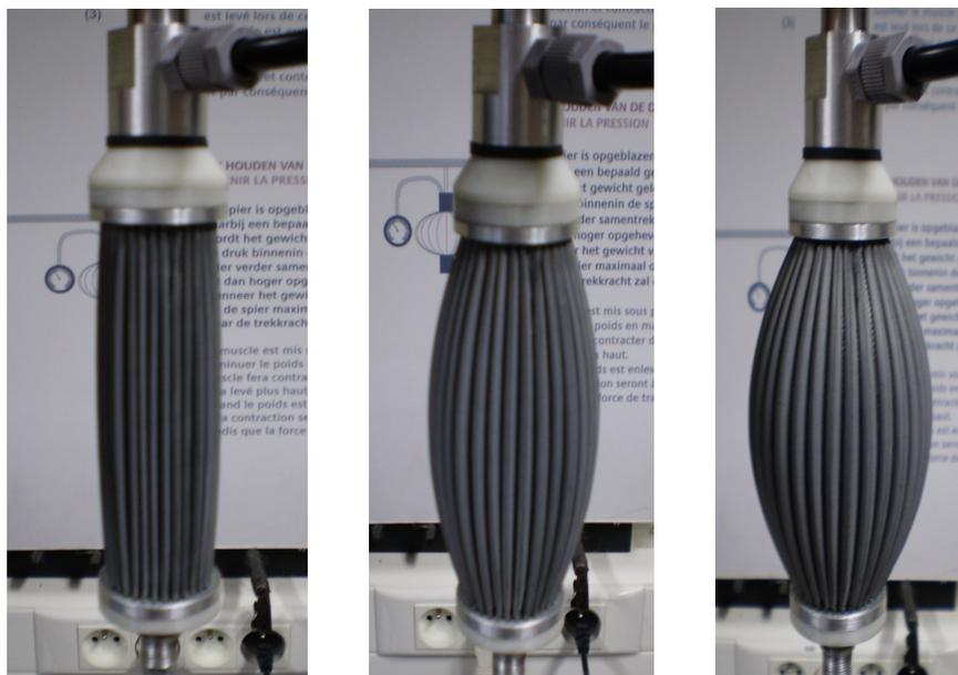
**Figure 3.21:** Photographs of the muscle prototypes at different states of inflation
