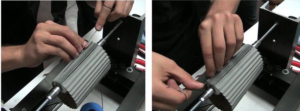
**Figure 3.20:** Photographs of the muscle body building process
