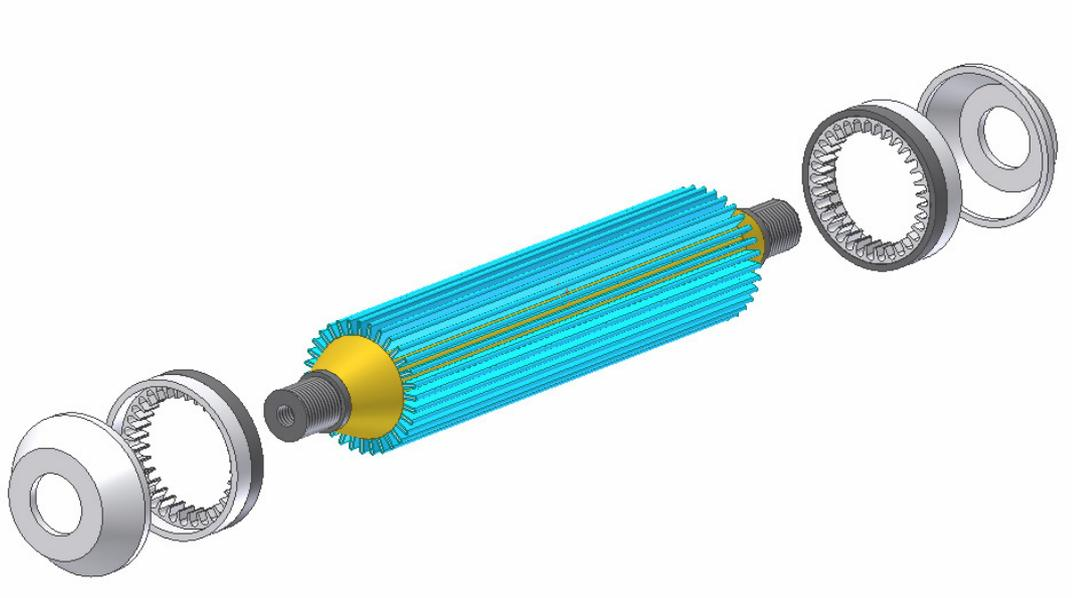
**Figure 3.10:** Composition of the new muscle prototype
