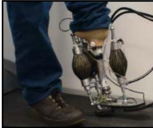
**Fig. 18: Powered Below-knee Prosthesis, using pleated pneumatic artificial muscles in order to generate ankle power (VUB). [22]**
